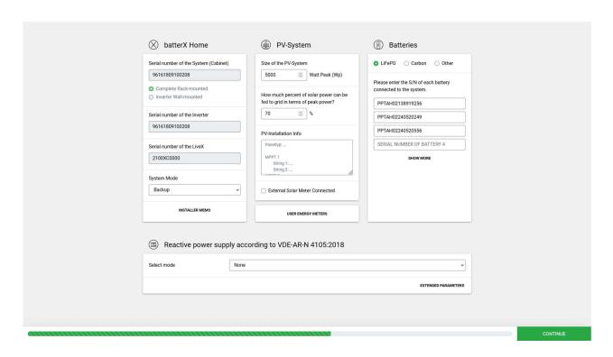
Our liveX energy management cloud offers multiple possibilities like time-delayed charging and adjustable backup power reserve. Detailed system analyses can be performed quickly.
