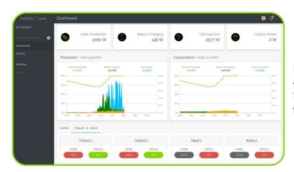
Live dashboard with energy flow diagram and display of all relevant parameters for the areas: Photovoltaics, battery system, grid and consumers.
