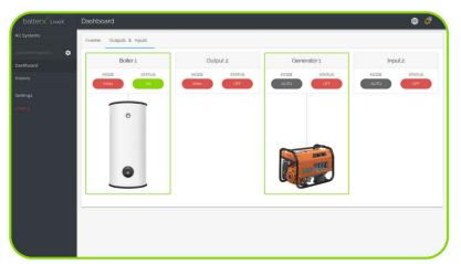
By means of an intelligent energy management system, programmable relay contacts can be used to control consumers such as a heat pump or a heating rod. This allows excess energy, which would otherwise be fed into the public grid, to be used intelligently in the house.
