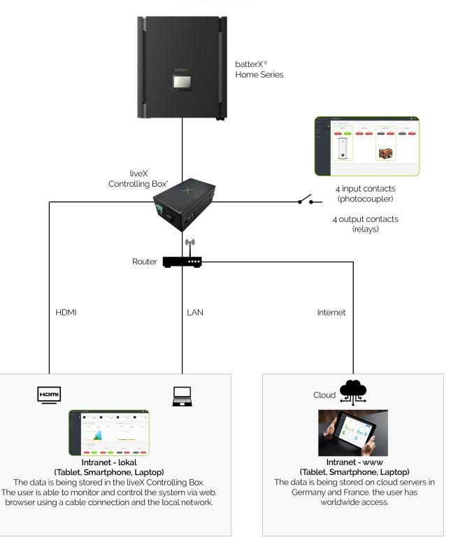
'Cloud-based monitoring and controlling: also availabe for local networks for monitoring and controlling, with adjustable feed-in limitation (Example: German EEG 70%). 8 programmable contacts for controlling external devices, such as load or generators, 4 input dry contacts and output relay contacts are available to be programmed in the liveX monitoring
