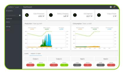
Live-dashboard with energy flow diagram and indication of all parameters: PV, battery, grid, consumption.
