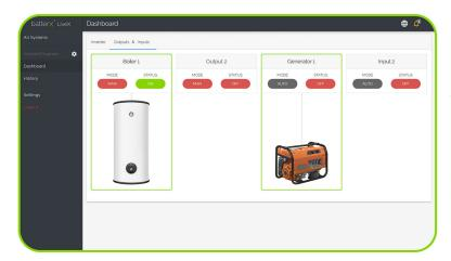
Activating programmable relay contacts the energy management tool becomes smart. Hereby it's possible to communicate with several energy sources like a diesel genset and loads which can be switched on or off depending on the customer requirement.
