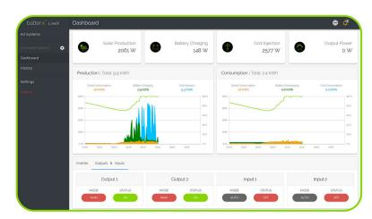
Live-dashboard with energy flow diagram and indication of all parameters: PV, battery, grid, consumption.
